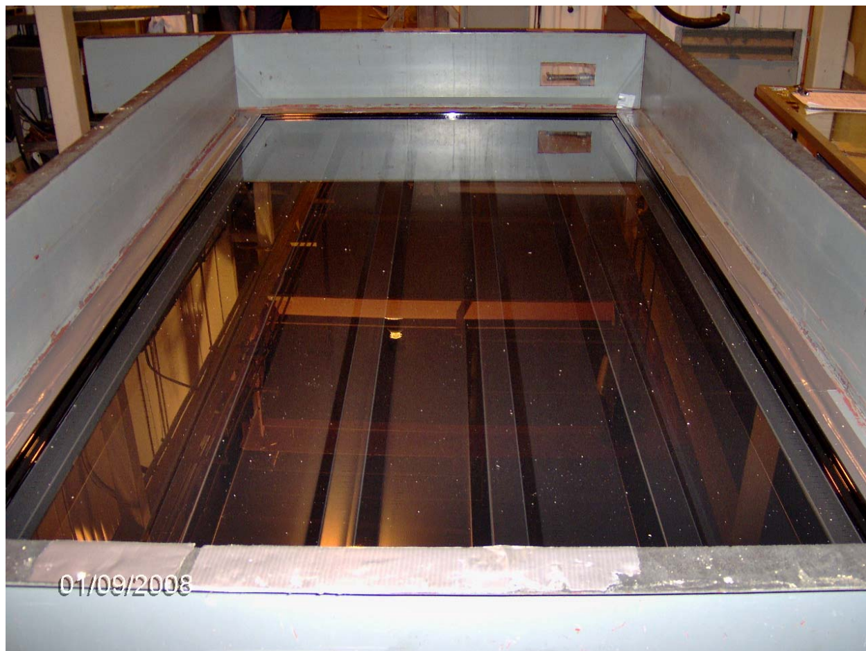
Figure 3: Top view (enclosure cover removed) showing tape seal around edges.
